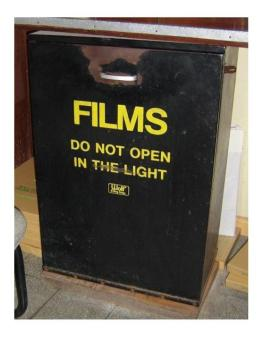
FIG. 24. Example of storage for unexposed X ray films. (Image courtesy of Chan Lai Kuan, Malaysia.)
