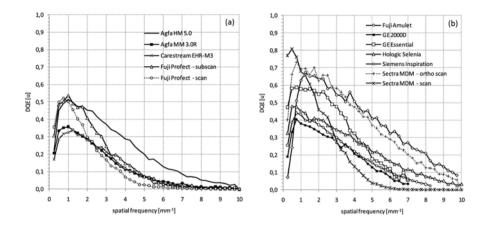
FIG. 44. DQE curves obtained using (a) CRM and (b) DDM systems. (Reproduced with permission from Marshall et al. [134].)
