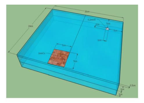
FIG. 41. Sample quality control phantom developed for remote and automated quality control in mammography (reproduced from Ref. [132]).
