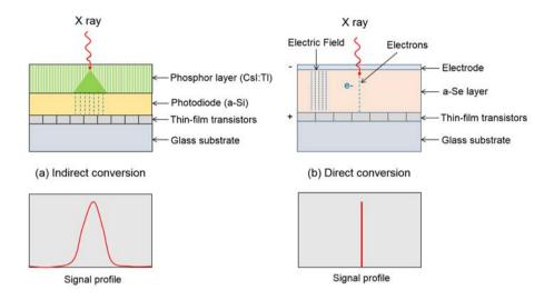
FIG. 35. Comparison of (a) indirect conversion and (b) direct conversion flat panel detector used in DDM systems.
