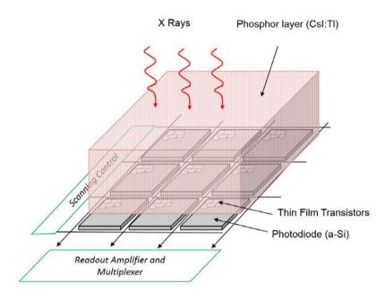
FIG. 34. Basic principles of an indirect conversion flat panel detector. Thallium activated caesium iodide (CsI:Tl) phosphor converts X rays into lights and then they are converted into charges by the amorphous silicon (a-Si) photodiode. The charges are stored in individual thin film transistors and then transferred to readout amplifiers and multiplexers to form a digital image.
