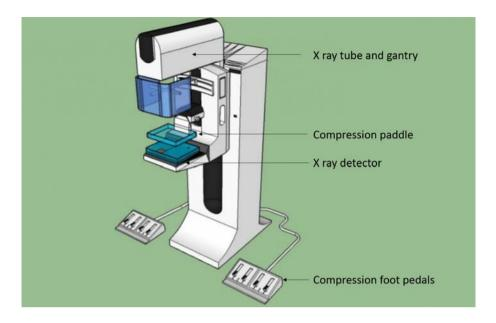
FIG. 9. Main components of typical mammography X ray equipment.
