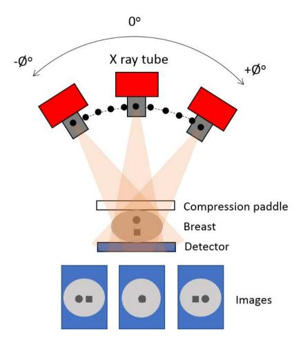
FIG. 39. Basic principle of DBT. The X ray tube moves over a limited angle  $(-\emptyset^{\circ} \text{ to } + \emptyset^{\circ})$ around the breast to acquire multiple projections. These projections are then reconstructed to produce a series of images in closely spaced focal planes parallel to the detector to overcome the issue of tissue overlapping in conventional 2-D mammography.
