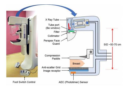
FIG. 32. Main components of a typical mammography X ray equipment.
