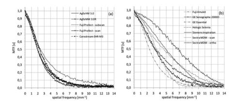
FIG. 42. MTF curves obtained from (a) CRM and (b) DDM systems. (Reproduced with permission from Marshall et al. [134].)
