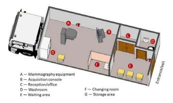
FIG. 29. Sample layout of a mobile mammography unit.
