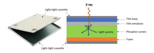
FIG. 21. Construction of a mammography screen-film system (single-emulsion single-screen combination).
