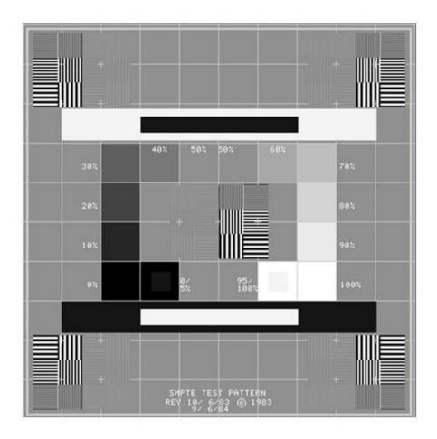
FIG. 19. Standardized Society of Motion Picture and Television Engineers test pattern, one type of test pattern that may be provided with the medical diagnostic monitor for quality control.
