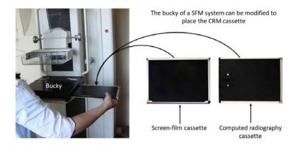
FIG. 26. A bucky from an SFM system can be modified to house the CR cassette without replacing the entire mammography set-up. (Photo courtesy of Konstantopoulio General Hospital, Greece.)
