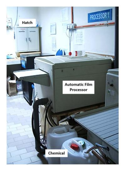
FIG. 23. Sample layout of a room for an automatic film processor. (Image courtesy of Chan Lai Kuan, Malaysia.)
