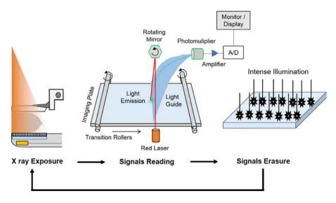
FIG. 36. Basic operations of a CR plates reader.
