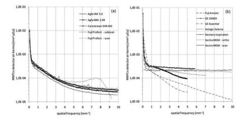
FIG. 43. Normalized noise power spectrum curves obtained using (a) CRM and (b) DDM systems. (Reproduced with permission from Marshall et al. [134].)
