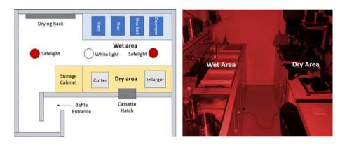
FIG. 22. Typical darkroom layout. (Image courtesy of Chan Lai Kuan, Malaysia.)
