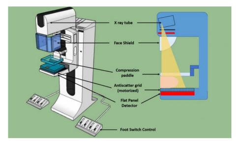
FIG. 12. Main components of DDM X ray equipment.
