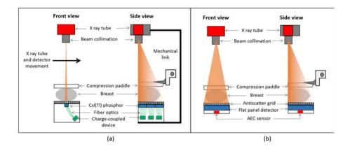
FIG. 33. Comparison of (a) a scanning detectors system and (b) an area detector system of a typical DDM system.
