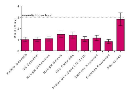
FIG. 45. Sample overview of the MGD to the 60 mm PMMA stack to reach the achievable limit of the 0.1 mm gold disc. Adapted from the United Kingdom National Health Service [139].
